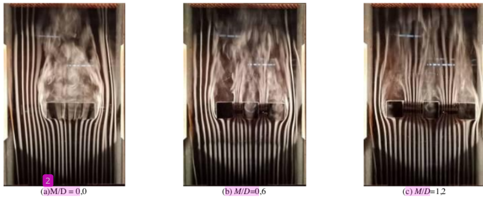
Figs. 9. Visualization of flow of three tandem square cylinder parallel in parallel configuration model II or (a) M/D and N/D=0.0 ; (b) M/D and N/D=0.6 and (c) M/D and N/D=1.2 at Re=43,844
